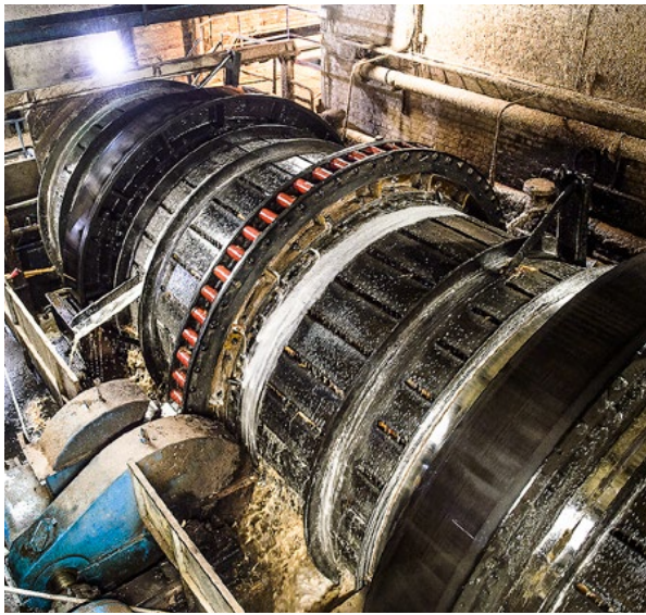
The logs rotate in a debarking drum to peel off the bark.
