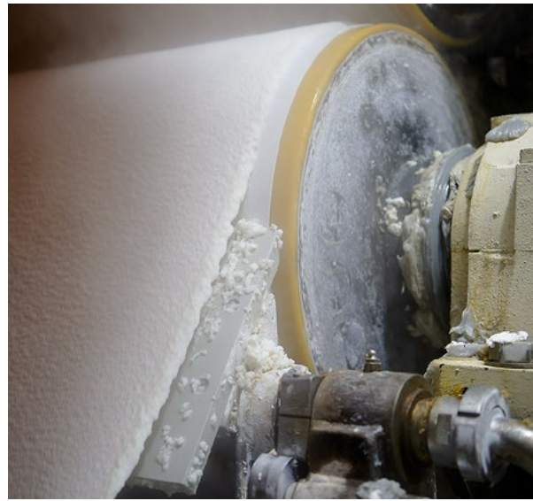
In the wet machine water is pressed out of the fiber web.
